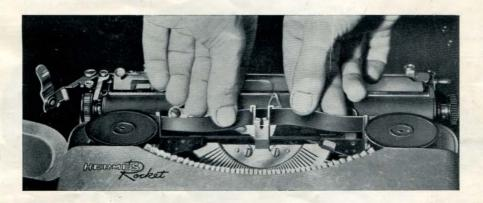
Now pass the ribon between the platen and the ribbon lifter and insert it **from behind** (see small illustration) and not from the front, through the slots on the left and right of the ribbon lifter (2). Shift lock (2) may then be released.
