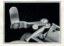
first character of the line, and sliding the left hand margin stop to the right until it stops automatically. Then move the carriage to the position where the line is required to finish, and slide the right hand margin stop to the left until it stops automatically.
